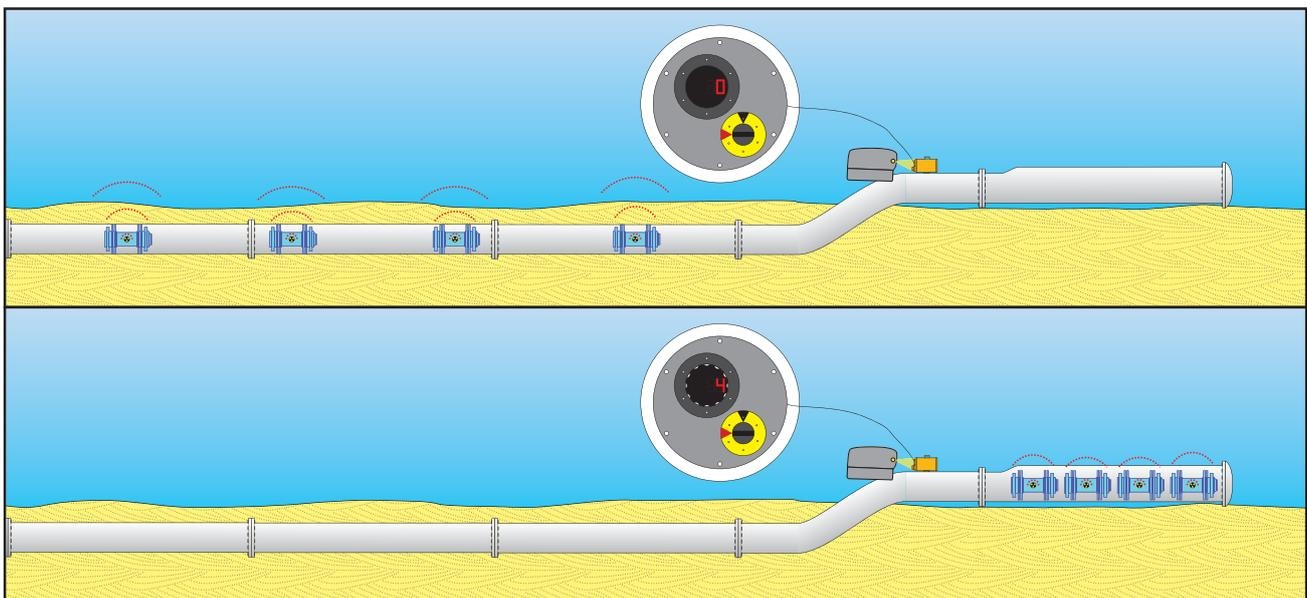
The PSU is positioned by a remotely operated underwater vehicle (ROV) to any location on the pipeline to count and confirm the transit of one or multiple pigs.
