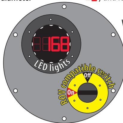
When a pig transit is detected, ultrabright white LEDs switch on for 5 seconds. Every 30 seconds the same white LEDs flash once for each pig transit. The flashes assist with pig counting when ROV visibility of the display is compromised due to water turbidity.
