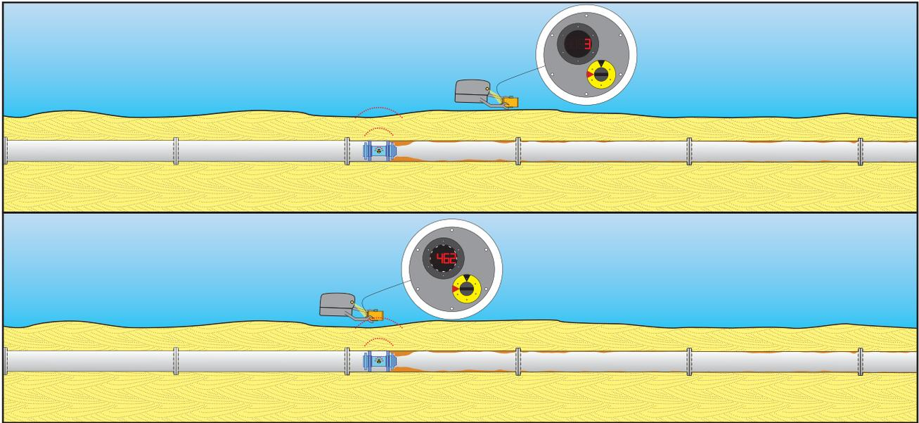
The PSU is transported by the ROV along the buried pipeline to identify the precise location of missing or stuck pigs.
